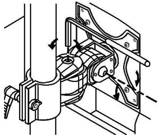
Adjusting the torque
