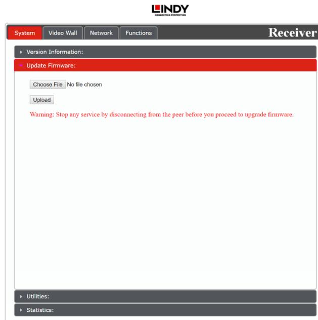
Provides a way to update the Receiver's firmware. Click "Choose File" to select the firmware update file from the local PC (\*.bin format). After selecting an appropriate file, click the "Upload" button to begin the update process.
