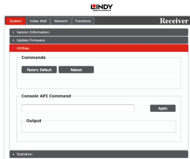
The Utilities window allows users to reset the unit back to the factory defaults by clicking "Factory Default". The unit may be rebooted (without resetting settings) by pressing the "Reboot" button.
