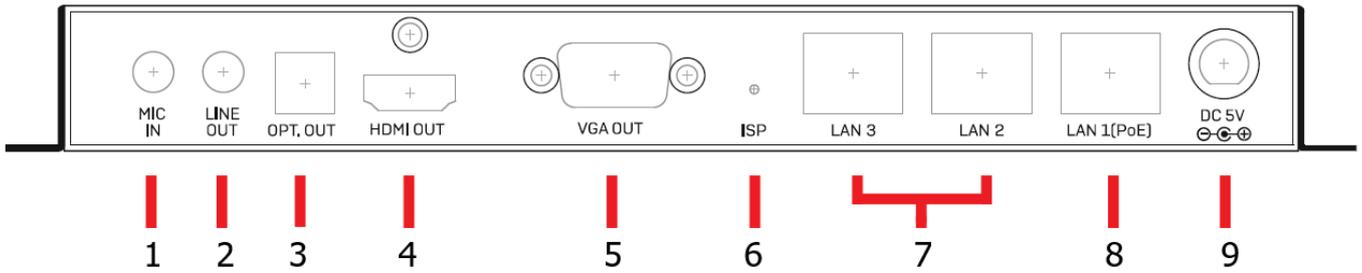
1. **MIC IN** – In a point to point installation connect a standard Microphone to send audio to the line out port of the transmitter (active only when an analog source is connected to the Line In port of the receiver).
