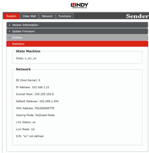
The Statistics window shows all available information about the operational status of the unit, including current Host ID Name, Ethernet information, MAC address, unicast/multicast mode, link status and mode.
