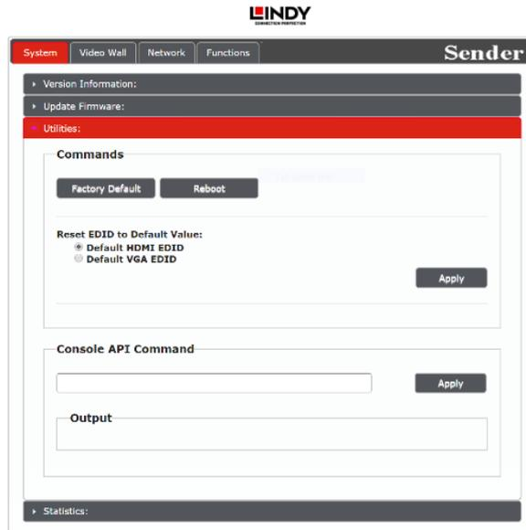
The Utilities window allows users to reset the unit back to the factory defaults by clicking “Factory Default”. The unit may be rebooted (without resetting settings) by pressing the “Reboot” button.
