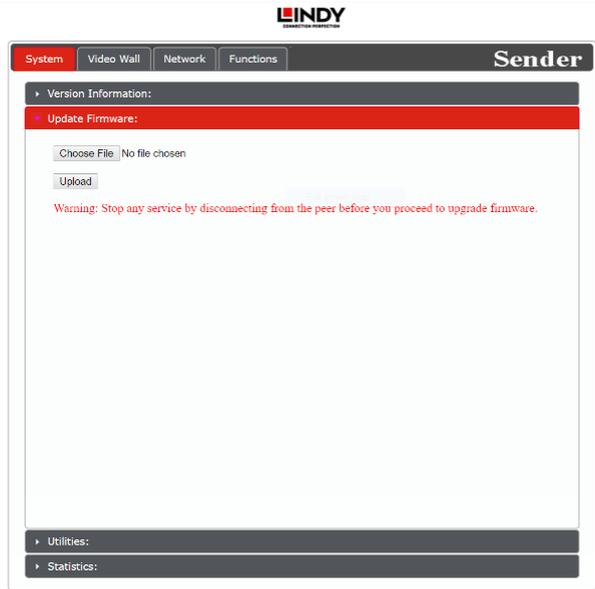
Provides a way to update the Transmitter's firmware. Click "Choose File" to select the firmware update file from the local PC (\*.bin format). After selecting an appropriate file, click the "Upload" button to begin the update process.
