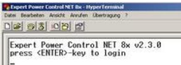
The power ports can be toggled by pressing numerical keys in the terminal program. The character "Z" will show the network settings. To logout, press the Esc key.
