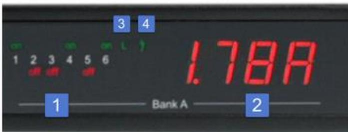
1. 6 plain text displays (on/off) for the state of the outputs (Bank A or B)
